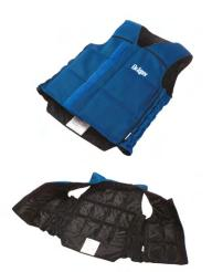
The Dräger comfort vest CVP 5220 helps to absorb excess body heat and offers comfort for the wearer when working in high temperature surrounding or performing tasks that are physical enough to cause perspiration. It can be worn underneath all forms of protective clothing. Its cooling action is derived from 20 PCM elements (Phase Change Material) integrated into the cool vest.
